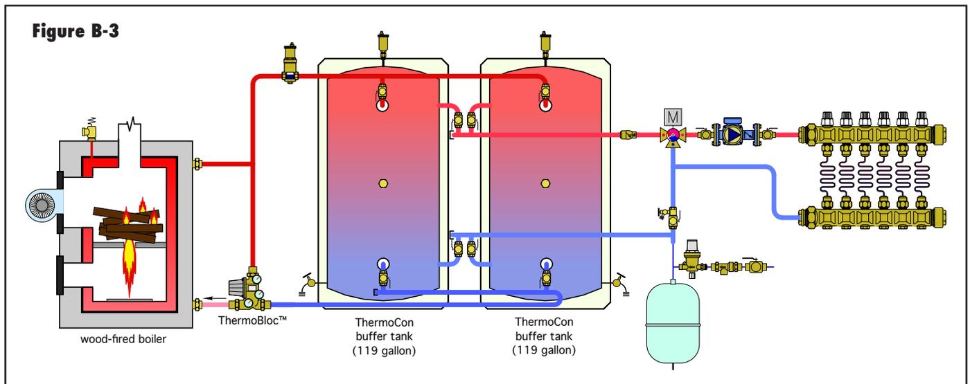
Discussion: This expansion tank volume is “conservatively” large because it assumes that all water in the system reaches the upper temperature of 200°F simultaneously. This is not the case for piping downstream of the mixing valve (e.g., the radiant panel circuits). Thus, it is not necessary to add any additional safety factor to this volume.
