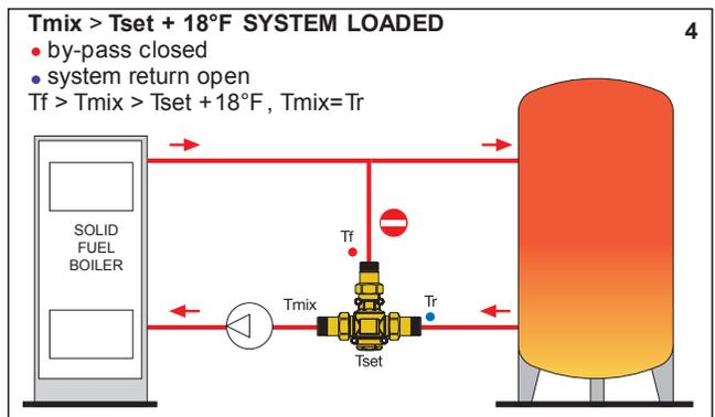
$T_f$  = Bypass flow from boiler
