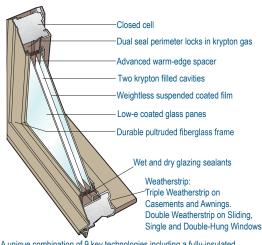
A unique combination of 9 key technologies including a fully-insulated fiberglass frame, suspended film, and gas-filled cavities maximize performance.
