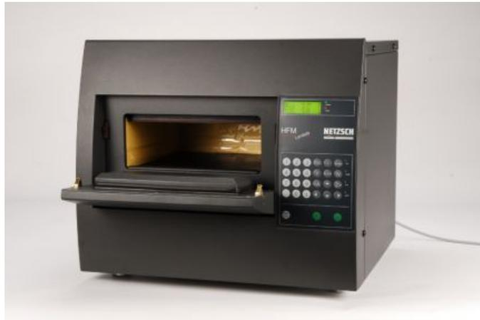
**The job requires special equipment.** Measuring a material's R-value according to the ASTM C518 test procedure requires a heat flow meter like this German appliance manufactured by Netzsch-Gerätebau. After a sample is placed between a hot plate and a cold plate inside the calibrated testing apparatus, the heat flow occurring at a defined temperature difference is measured with a heat flux sensor.
