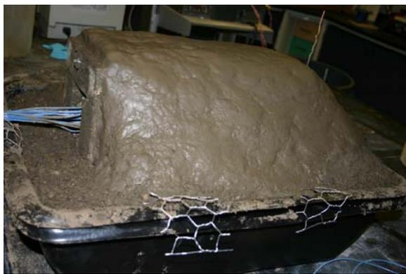
Figure 4: Scale model ECM with earth covering.
