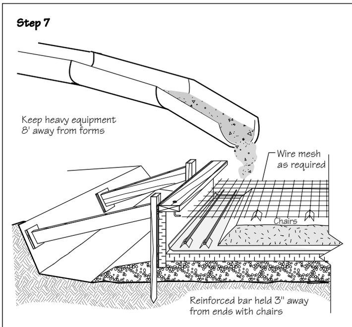
**Step 7: Place Reinforcing Steel, Wire Mesh (as required) and Pour Concrete**
