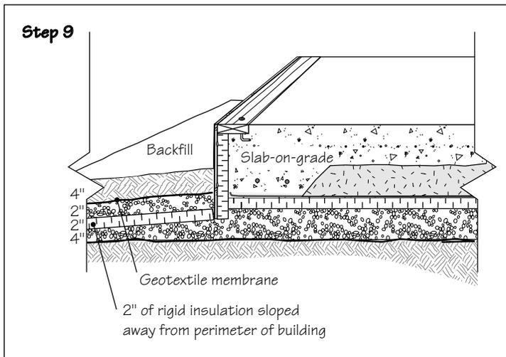
**Step 9: Insulate Horizontal Trench Adjacent to the Building and Backfill**
