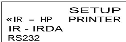
The Printer Setup Screen is displayed by repeatedly pressing the **MENU** key from the Combustion Test Screen. Use this screen to choose the type of connection and printer being used.
