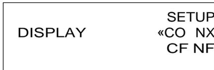
The Display Setup Screen is displayed by repeatedly pressing the **MENU** key from the Combustion Test Screen. Use this screen to select whether the Combustion Test Screen will display the measured values of Carbon Monoxide and Nitric Oxide (CO and NX), or the calculated values of these gases (CF and NF) referenced to Oxygen.
