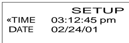
The Time/Date Setup Screen is displayed by repeatedly pressing the **MENU** key from the Combustion Test Screen. Use this screen to enter the current time and date as follows:
