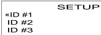
This initial ID Setup Screen is displayed by repeatedly pressing the **MENU** key from the Combustion Test Screen. Use this screen to edit three lines of customer information (e.g., the customer's name, location, and burner reference number).
