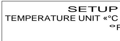
The Temperature Setup Screen is displayed by repeatedly pressing the **MENU** key from the Combustion Test Screen. Use this screen to setup the analyzer to display temperature in either  $^{\circ}\text{C}$  or  $^{\circ}\text{F}$ .
