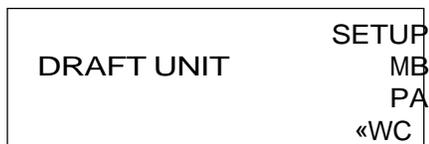
The Draft Unit Setup Screen is displayed by repeatedly pressing the **MENU** key from the Combustion Test Screen. Use this screen to setup the analyzer to display draft in either millibars (MB), Pascals (PA), or inches-of-water column (WC).
