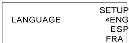
The Language Setup Screen is displayed by repeatedly pressing the **MENU** key from the Combustion Test Screen. Use this screen to select the language displayed on the analyzer. The languages available for selection include English (ENG), Spanish (ESP), and French (FRA).
