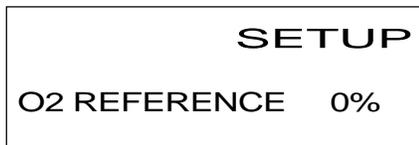
The O<sub>2</sub> Reference SETUP Screen is displayed by repeatedly pressing the **MENU** key from the Combustion Test Screen. Use this screen to select the O<sub>2</sub> reference level that the analyzer will use to calculate the CO and NX gas levels as referenced to Oxygen.
