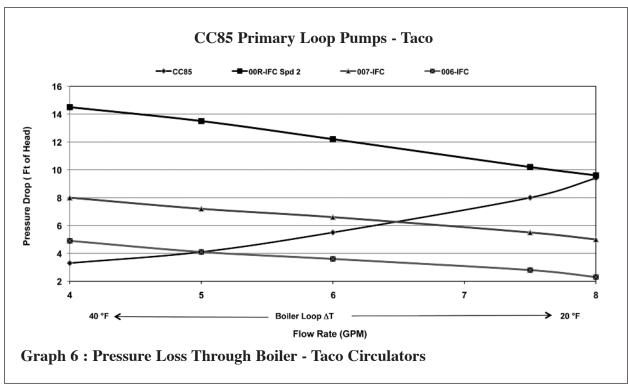
Minimum allowable boiler flow rate at full input: 4 gpm [15 lpm] CHALLENGER CC85
