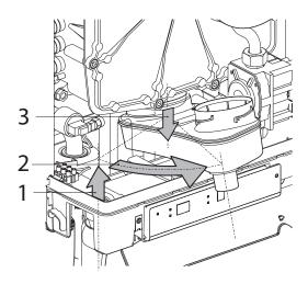
Fig. 25: Removal of Condensate Pan
