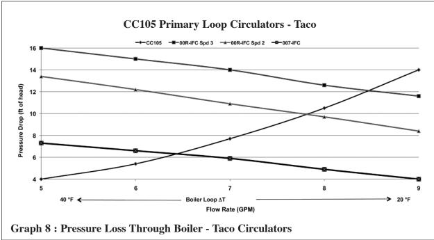
Minimum allowable boiler flow rate at full input: 5 gpm [19 lpm] CHALLENGER CC105
