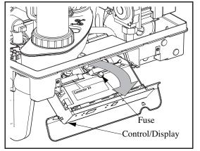
Fig. 17: Accessing Low Voltage X4 Connections
