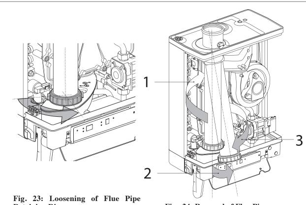
Fig. 23: Loosening of Flue Pipe Retaining Ring
