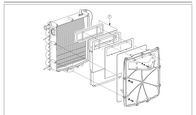
Fig. 32: CHALLENGER Burner Components
