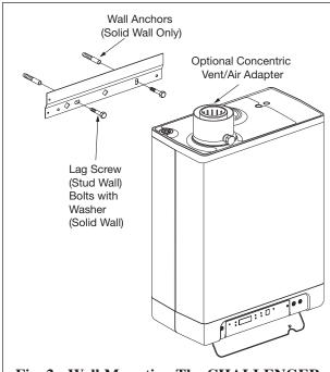
Fig. 2: Wall Mounting The CHALLENGER
