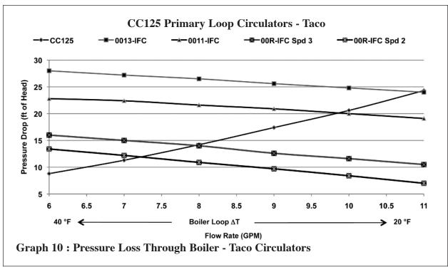
Minimum allowable boiler flow rate at full input: 6 gpm [23 lpm] CHALLENGER CC125
