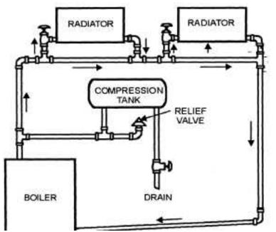
A tank with its vent open to the atmosphere is installed in the system above the highest radiator for water expansion. The water level in the expansion tank rises and falls, as the system is heated and cooled, and the system is full of water and free from air at all times. In the open-tank gravity hot-water heating system, the expansion tank is installed on a riser directly above the boiler, so the air liberated from the boiler water enters the tank and is not retained in the system.
