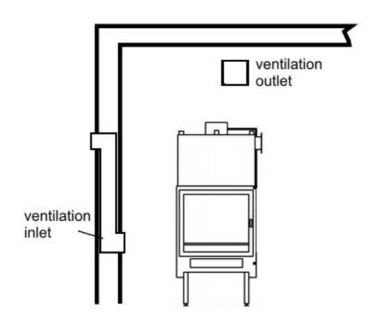
Natural chimney draught generated by chimney institutes the basis of correct of fireplace. If it is too low can cause the flue gases regress to room and too high draught accelerates the process of combustion, which leads to quicker burning of fuel and can cause non-controlment raise of temperature of factor in water jacket.
