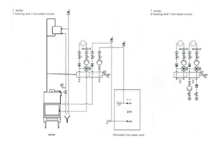
It happens often that existing installations are secured by closed arrangement. Unless we have the possibility of opening of installation we can then protect fireplace with open installation arrangement and connect across plate exchanger to closed arrangement.
