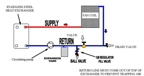
WARNING: Install the water-to-air heat exchanger on the warm-air side of the central furnace fan. Installing the exchanger on the cold-air return inlet may overheat
