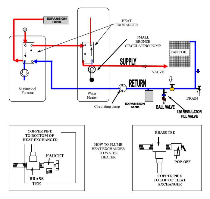
**WARNING:** Install the water-to-air heat exchanger on the warm-air side of the central furnace fan. Installing the exchanger on the cold-air return inlet may overheat components of the furnace and cause them to operate other than as intended.
