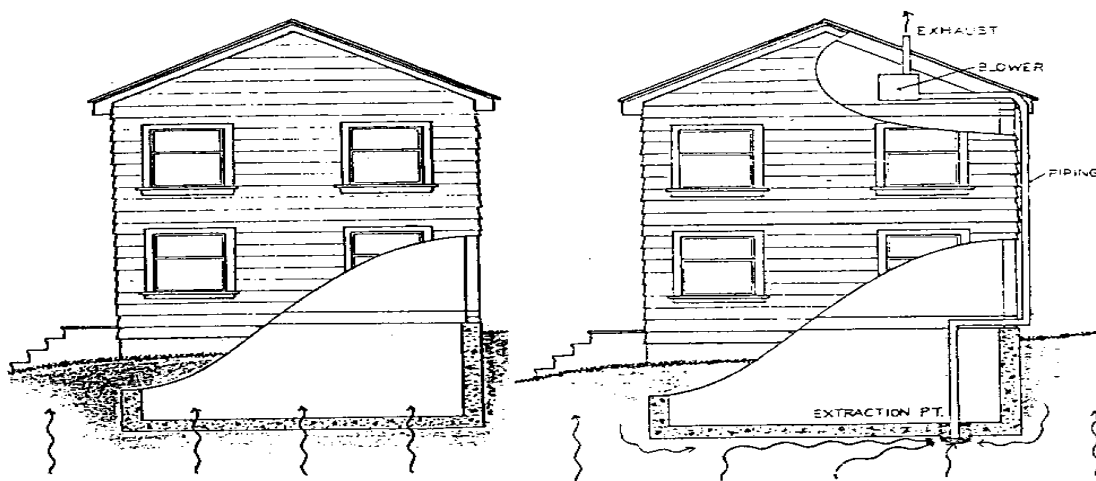
Figure 1 - Schematic Diagram of Typical Residential SSD System
