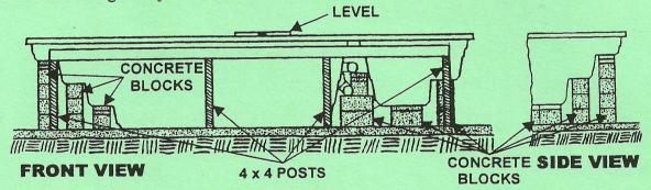
All **AQUASWIM'N'SPAS**<sup>TM</sup>, whether installed above ground, inground, or partial inground must be supported from under the wall stiffener with 4" x 4"s along each side (as shown).
