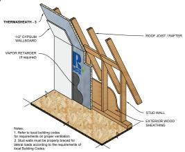
Attics and Crawl Spaces - Thermasheath-3 may be applied to the interior face of stud walls or roof rafters within attics and crawl spaces to provide a layer of continuous insulation (ci). Simply nail the Thermasheath-3 to the framing members and cover with an approved ignition barrier such as 3/8 inch gypsum wallboard or 1/4 inch wood structural panel, particle board or hardboard.
