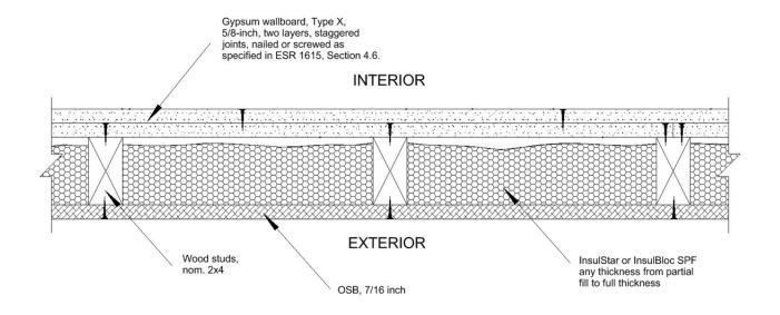
FIGURE 2 SYMMETRICAL ONE-HOUR FIRE RESISTANCE-RATED WALL ASSEMBLY
