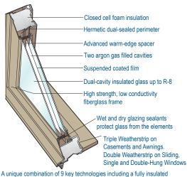
fiberglass frame, suspended film, and gas-filled cavities maximize
