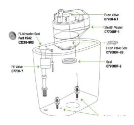
The Stealth dual flush toilet uses 0.5/0.95 gallons per flush. It is a vacuum assist toilet made by Niagara. We have installed these in all three bathrooms.
